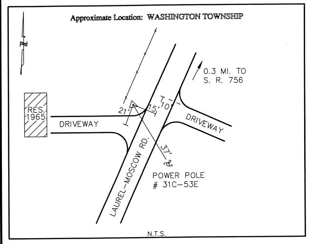
Azimuth: N 32° 10′ 53" E to Station 261.
