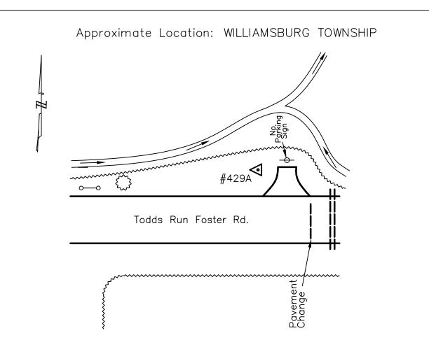
AZIMUTH: S.72°24'52"E. TO STATION 429
